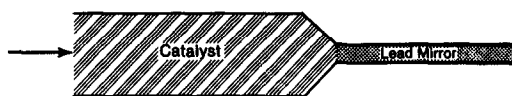
FIG. 7. Quartz reactor tube used for lead mirror experiments. The large diameter and tapered sections were inside the furnace, the small diameter section was outside.
